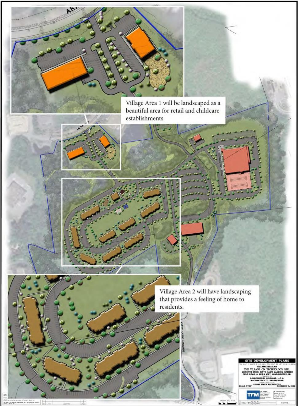
Figure 2.9.B.13-1: Village area 1 will be landscaped as a beautiful area for retail and childcare establishments. The residential area, Village area 2, will have landscaping that reduces heat islands and provides a feeling of home to residents. Parking lots will have landscaped medians with shade trees every 50 ft.
